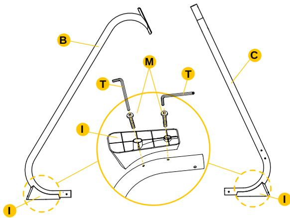
**TIPS:** Since the support feet are deep and the screws are short, use a hex wrench (T) to secure the screw heads before tightening the screws.
