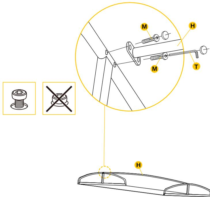
**TIPS:** To make installation easier, first bend the top support rod a little. Then install one side to align the screws first, and then install the other side.
